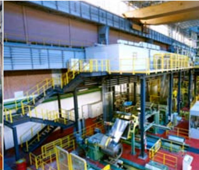
Bright Annealing with in-line tension leveling 1270 mm wide
